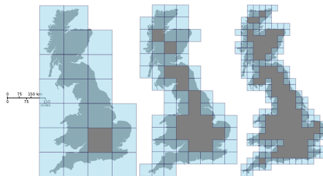
Figure 1: Example of estimating the box-counting dimension of the coast of Great Britain (source: Wikipedia).
