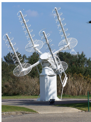
Array of four axial-mode helical antenna 18
