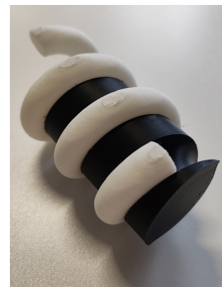
A helix on a cylinder with external thread.
